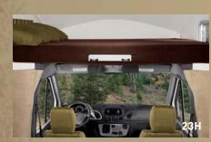
**Overhead Bunk.** Gas struts lift the hinged bunk out of the way during the day. At night, the bunk provides a spacious and comfortable 49inch x 75-inch sleeping space.
