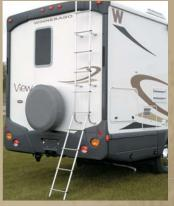
**Extension Ladder.** Our innovative ladder is mounted to the back wall with a folding design for quick use and storage.
