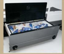
**Sliding Storage.** An easy-to-use sliding exterior storage bin seals tightly to protect your things from dirt and moisture. It even includes a drain plug that makes cleaning easier.
