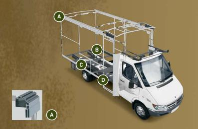
SUPERSTRUCTURE® is the term given to Winnebago Industries' structural motor home design and construction. Rather than a single component, it is the culmination of design integration that incorporates steel and aluminum substructures; welded tubular aluminum floor supports; interlocking joint technology; and Thermo-Panel® floor, roof and sidewalls to form a high-strength, durable vehicle body.
