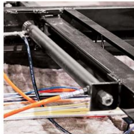
Commercial hydraulic rack & pinion slide-outs. All gear boxes are located inside the frame for the ultimate weather protection.
