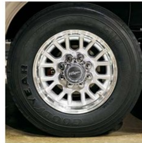
Heavy-duty 17.5" Goodyear® tires provide increased load capacity while staying cool on long hauls. We use truck tires, not RV tires, to ensure better performance and peace of mind.
