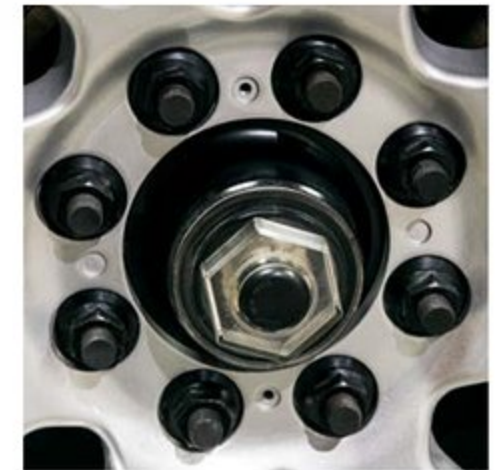
Commercial E-Z Lube® hubs surrounded by 8 large 5/8" stud bolts and standard automotive disc brakes round out the safety features of every DRV unit.
