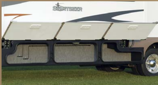
WEB STOREMORE No more crawling on your hands and knees, thanks to our exclusive slideout system that allows exterior compartments to extend with the slideroom for easy storage access.
