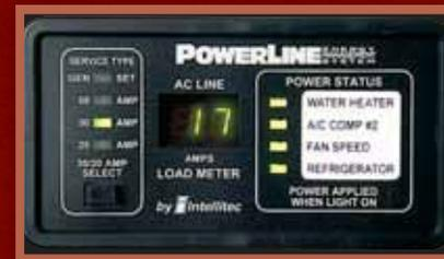
**WEB POWERLINE**® energy management system monitors electrical usage and automatically cycles appliances on and off to prevent tripped campground circuit breakers.
