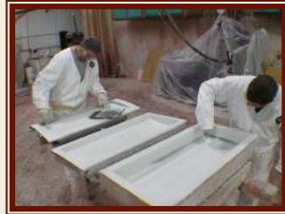
Fiberglass Fabricators...Preparing fiberglass body, fiberglass exterior storage boxes, fiberglass steps, and other components.
