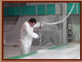
Fiberglass Fabricators...Preparing fiberglass body, fiberglass exterior storage boxes, fiberglass steps, and other components.
