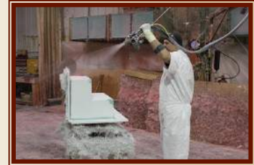
Fiberglass Fabricators...Preparing fiberglass body, fiberglass exterior storage boxes, fiberglass steps, and other components.
