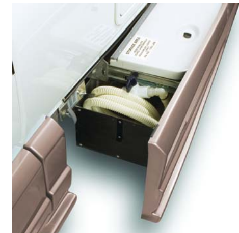
The macerator sewage pump on all models chops up any solids and tissue and ejects the entire contents through a convenient 1¼" hose. No mess, no fuss.
