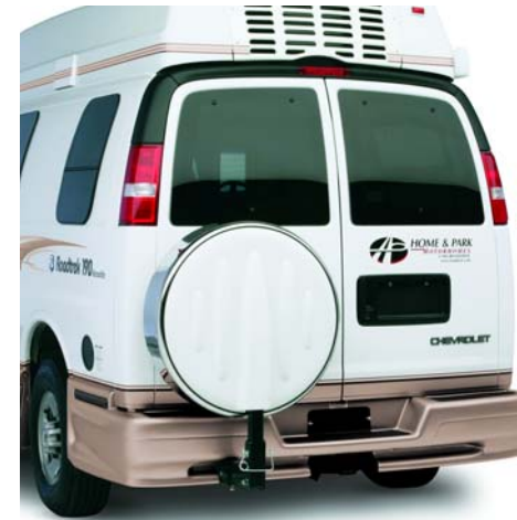
Optional Continental kit looks great and provides more interior storage. It's mounted on the receiver to avoid stress and rust on the door and off centre to the trailer hitch to allow towing and access to one door. To access the other door, simply remove the hinge pin to lower the spare tire. To access the tire, just unclasp the tire cover.
