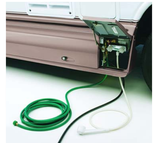
There is a separate compartment for an exterior shower and city water connection with quick disconnect. The 210 features a detachable power cord for trips away from the campsite.
