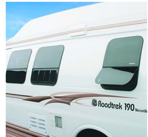
Frameless awning windows are better looking, reduce wind noise, improve aerodynamics, and provide superior air circulation even during foul weather. Their larger size provides a better view from inside. The Integrated Venting System ( 170 and 190 models ) provides inconspicuous ventilation of the refrigerator.
