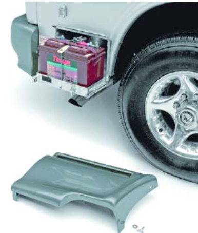
A large capacity auxiliary lead acid battery is totally concealed yet easily accessible on slide-out tray. A second auxiliary battery is optional on 190 and 210 models.
