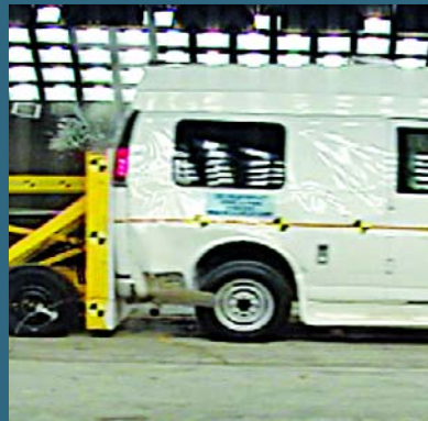
This photo shows the rear impact test. The test vehicle was impacted by a moving barrier at 30-mph (48 km/h). The entire fuel system was then inspected for leakage. Our test vehicle did not leak any fuel.
