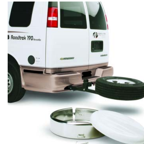
Optional Continental kit looks great and provides more interior storage. It's mounted on the receiver to avoid stress and rust on the door and off centre to the trailer hitch to allow towing and access to one door. To access the other door, simply remove the hinge pin to lower the spare tire. To access the tire, just unclasp the tire cover.
