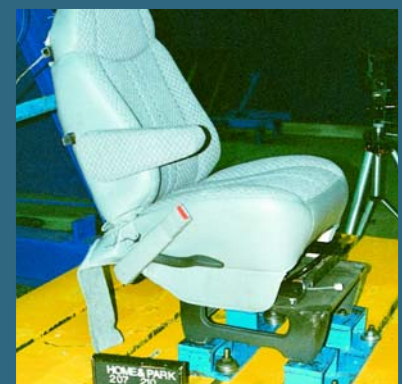
Seating system testing minimizes the possibility of failure of the seats, their attachments and their installation.
