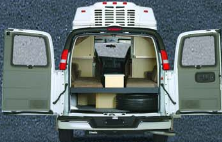
Dual rear doors allow for easy rear loading and swing a full 180° on 170 and 190 models and 270° on RS models.
