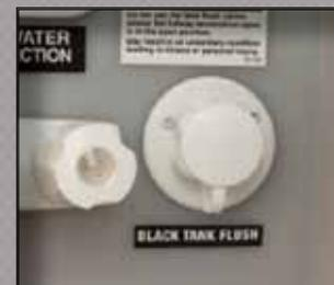
The black tank flush makes emptying the tank a clean, easy process!
